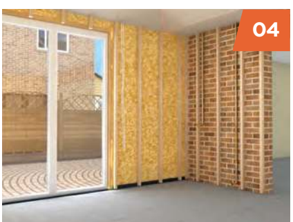
The interior has services added and is battened ready for internal finish.
